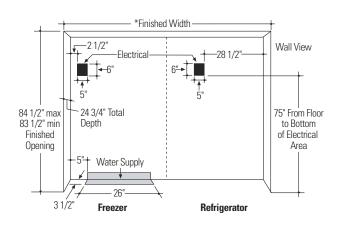
\*72" min. for a flush installation 71-1/2" min. for a semi-flush installation
